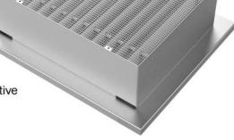
**WSG-H3** horizontal weather-proof louvre for supply and exhaust air Frame made of 3 mm thick aluminium profiles bent at the edges and continuously seamwelded, frame depth 320 mm. Upper contact flange flush, standard flange width 150 mm. Inner circumferential drip rail 50 mm and drains at the bottom for water removal.
